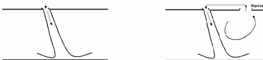
Figure 5 Air curtain without (left) and with (right) recirculating flow
