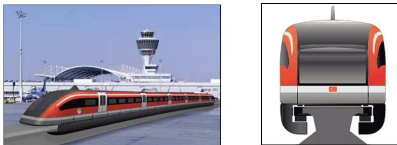
Figure 1: An artist impression of the magnetic levitation rail link (MAGLEV) at the airport in Munich and the layout of the guideway (Illustration of BMG)
